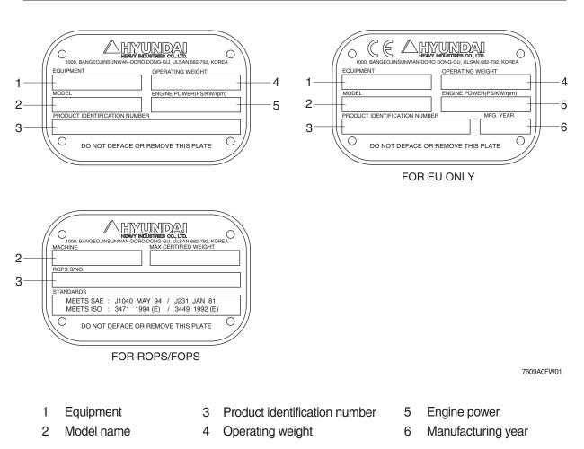
\* The product identification number (machine serial number) assigned to this particular machine and should be used when requesting information or ordering service parts for this machine from your authorized HYUNDAI dealer. The product identification number is also stamped on the frame.
